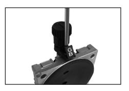
Loosen connection fastener slightly.
