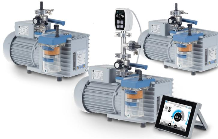
The RZ 2.5 and RZ 6 rotary vane pumps are available as useful packages with FO filter for oil mist separation (with integrated pressure relief valve) and manual in-line solenoid valve to reliably warm up the pump. A package with additional vacuum gauge VACUU·VIEW extended for fine vacuum is also an option.
