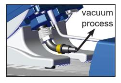
Connect the vacuum connection of the controller (measurement connection at the rear of the CVC 3000; hose nozzle for tubing I.D. 1/4" / 3/8" (6 / 10 mm) or connection for PTFE tube I.D. 3/8", O.D. 5/16" (10 / 8 mm)) via hose or PTFE tubing to the vacuum application. The cross-section of the tubing should be as large as possible.
