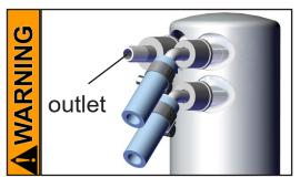
Never block the gas outlet (hose nozzle for tubing I.D. 3/8" (10 mm)). The exhaust hose has always to be unobstructed and without back pressure to enable an unhindered discharge of gases and protect the pump valves from damage.
