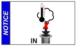
Avoid overheating (e.g., due to hot process gases). Maximum permissible temperature range: see "Gas inlet temperatures", pg. 30.
