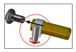
Secure hose connections at the pump appropriately, e.g., with hose clamps, to protect against accidental detachment.
