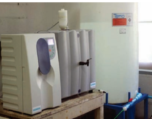
▲ A point-of-use modular water system. Tap feed RO/EDI system provides Type II quality water, but will achieve 10 Megohms consistently.
