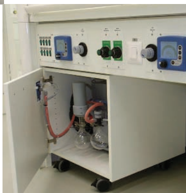
◀ With local vacuum pumping systems, the pump fits under a fume hood, with manual or electronic vacuum controls mounted on the fume hood panels.
