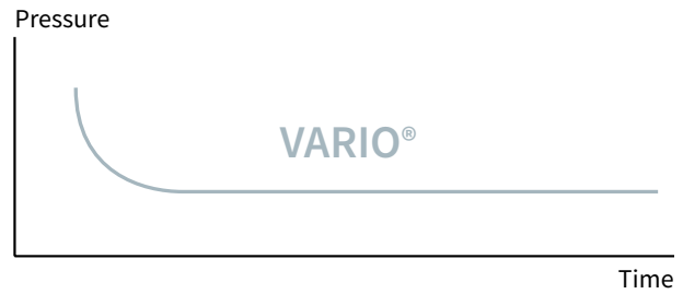
Fig. 20: Pinpoint regulation via speed control
