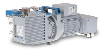
The RC 6 chemistry-HYBRID pump is the optimized corrosion resistant combination of a two-stage rotary vane pump and a chemistry diaphragm pump. The diaphragm pump continuously maintains the oil reservoir of the rotary vane pump under vacuum and prevents condensation in the oil-sealed part under corresponding pressure and temperature conditions.
