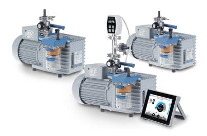
The RZ 2.5 and RZ 6 rotary vane pumps are available as useful packages with FO filter for oil mist separation (with integrated pressure relief valve) and manual in-line solenoid valve to reliably warm up the pump. A package with additional vacuum gauge VACUU-VIEW extended for fine vacuum is also an option.
