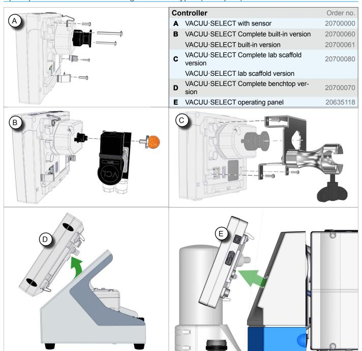
Disassembly / Disposal / Installation
