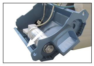
18. Unscrew the motor capacitor.
