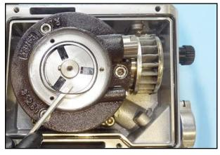
23. Remove the seal on the bearing cover.
