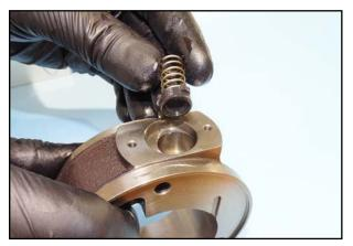
60. Insert a new cap and spring into the stator.
