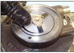
23. Pull the vanes and springs out of the rotor.
