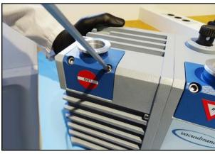
112. Unscrew the small flange connections at the inlet and the outlet.
