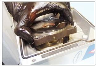
35. Remove the bearing plate from the housing.
