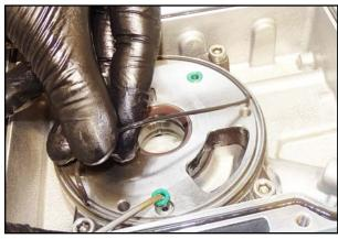
39. Remove the seals on the bearing plate.
