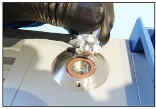
106. Remove the gas ballast connection.
