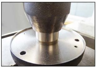
55. Press the shaft seal into the bearing cover as far as it will go.
