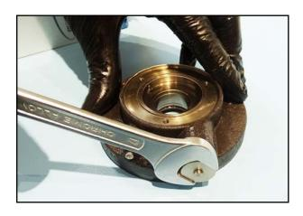
38. Unscrew the screw plug of the oil retention valve from the bearing cover.
