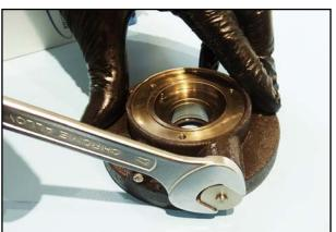
45. Unscrew the screw plug of the oil retention valve from the bearing cover.
