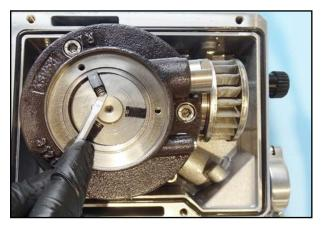
24. Pull the vanes and springs out of the rotor.
