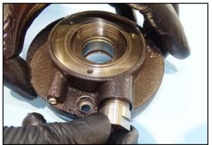
72. Screw the retaining device into the bearing cover.
