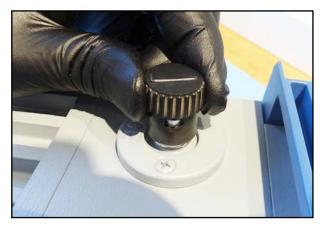
103. Remove the gas ballast cap.
