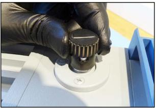
116. Remove the gas ballast cap.
