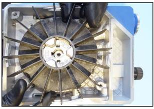
23. Insert the fan wheel with the coupling and push the fan wheel in as far as it will go.
