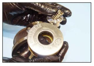
48. Remove the screw and the spring.
