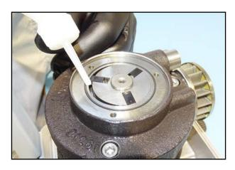
93. Fill the space around the rotor with the vacuum pump oil with which you operate the pump.
