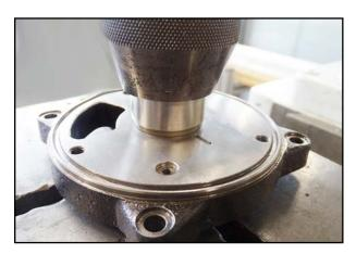
59. Press the shaft seal into the bearing plate as far as it will go.
