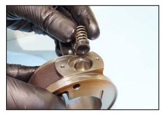
67. Insert a new cap and spring into the stator.
