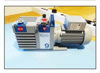
130. Let the pump run for approx. 1 hour with the outlet open, the gas ballast valve open and the inlet closed.
