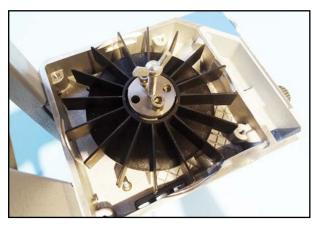
9. Place the pull-off disk on the coupling and insert the wing screw and the two cylinder screws.
