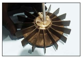
13. Remove the pull-off disk and the screws from the fan wheel.
