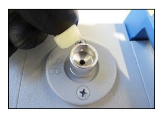
117. Remove the insulating material from the gas ballast connection.
