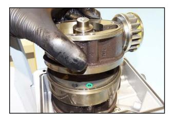
30. Lift off the stator.
