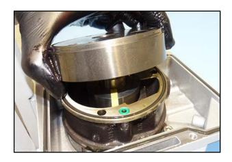
34. Remove the intermediate bearing.
