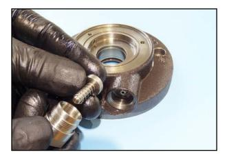
71. Assemble the oil retention valve with housing.
