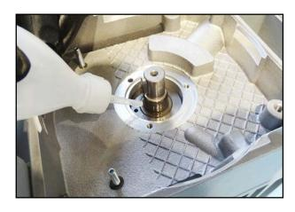
98. Turn the pump and fill the space in front of the removeable sleeve with the vacuum pump oil with which you operate the pump.
