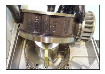
30. Lift off the stator.
