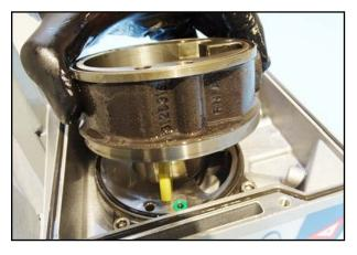
36. Lift off the stator.
