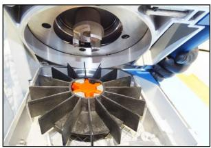
96. Carefully place the motor in the housing.
