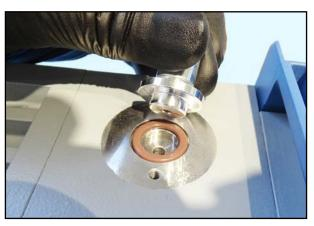
120. Remove the gas ballast connection.
