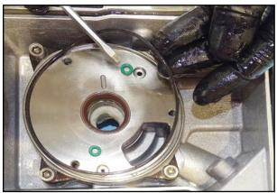
33. Remove the seals on the bearing plate.
