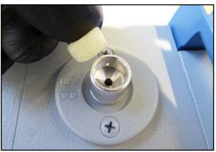
104. Remove the insulating material from the gas ballast connection.
