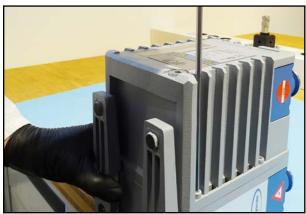
19. Loosen the screws on the oil reservoir.
