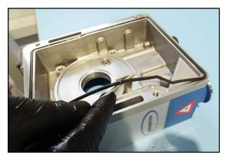
44. Remove the oil reservoir seal.
