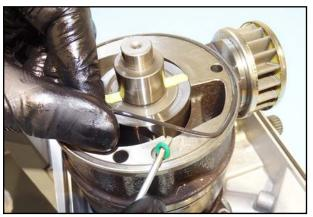
29. Remove the seals on the stator.
