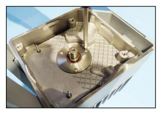
16. Unscrew the removeable sleeve.
