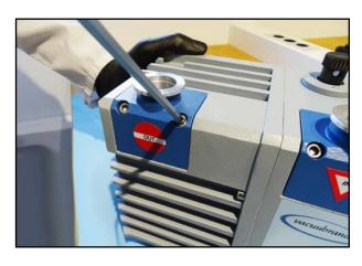
99. Unscrew the small flange connections at the inlet and the outlet.
