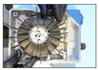
93. Insert the fan wheel with the coupling and push the fan wheel in as far as it will go.
