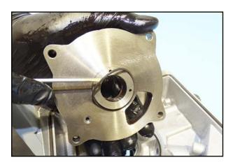
42. Remove the seal at the bearing plate.
