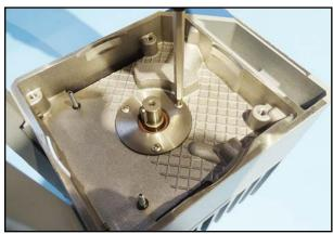
14. Unscrew the removeable sleeve.
