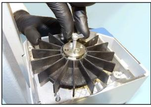
11. Screw in the wing screw until the fan wheel with coupling is released.
