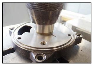
66. Press the shaft seal into the bearing plate as far as it will go.
