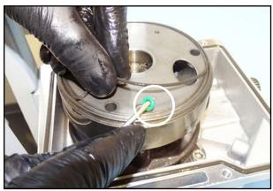
33. Remove the seals on the intermediate bearing.
