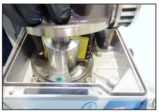
73. Press the vanes together and insert the stator.
