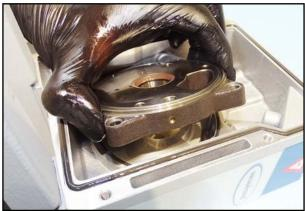
41. Remove the bearing plate from the housing.
