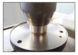
62. Press the shaft seal into the bearing cover as far as it will go.
