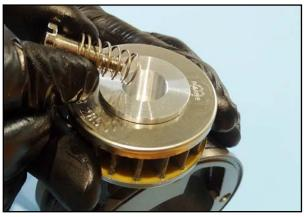
70. Insert the oil separator and tighten the oil separator with the spring and the screw.
