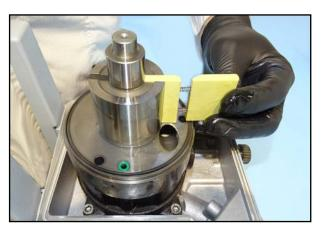
84. Insert the vanes with springs into the rotor.
