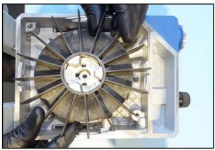
106. Insert the fan wheel with the coupling and push the fan wheel in as far as it will go.
