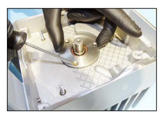
15. Lift off the removeable sleeve.
