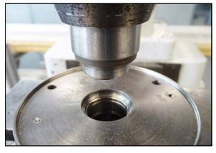
61. Place the shaft seal on the press-fit mandrel.
