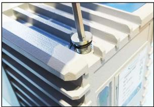
129. Screw in the oil inlet screw.
