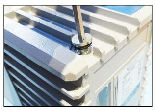
115. Screw in the oil inlet screw.
