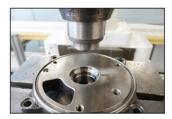
65. Place the shaft seal on the press-fit mandrel.
