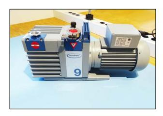
116. Let the pump run for approx. 1 hour with the outlet open, the gas ballast valve open and the inlet closed.
