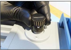
126. Insert the gas ballast cap.
