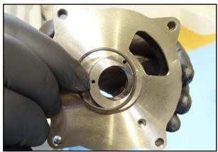
74. Place the O-ring around the bearing plate.
