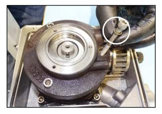
76. Insert the screws with Usit rings into the holes in the bearing cover.
