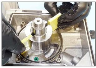
31. Pull the vanes and springs out of the rotor.
