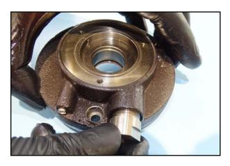
65. Screw the retaining device into the bearing cover.
