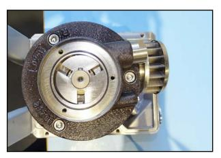
91. Be sure to place the oil pump rotor in the bearing cover so that the chamfer is on the side of the bearing cover.
