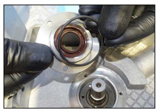
16. Place a new O-ring around the new removeable sleeve.
