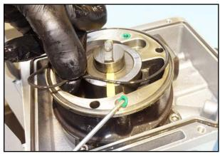
35. Remove the seals on the stator.
