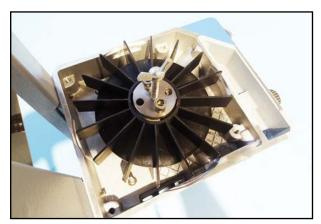
7. Place the pull-off disk on the coupling and insert the wing screw and the two cylinder screws.
