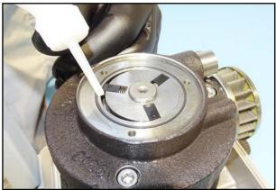
81. Fill the space around the rotor with the vacuum pump oil with which you operate the pump.
