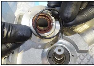
99. Place the O-ring around the new removeable sleeve.
