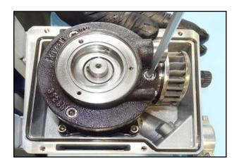
26. Unscrew the screws on the pump unit.
