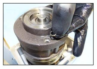
88. Insert the screws with Usit rings into the holes in the bearing cover.
