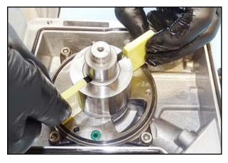
72. Insert the vanes with springs into the rotor.
