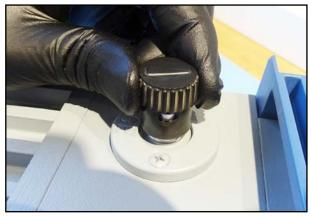
112. Insert the gas ballast cap.
