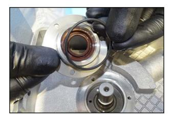
86. Place the O-ring around the new removeable sleeve.
