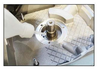
85. Turn the pump and fill the space in front of the removeable sleeve with the vacuum pump oil with which you operate the pump.
