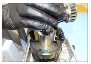
85. Press the vanes together and insert the stator.
