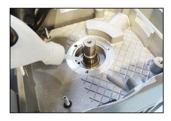
17. Fill the space in front of the removeable sleeve with the vacuum pump oil with which you operate the pump.
