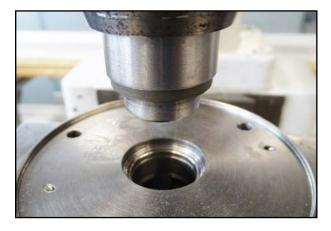
54. Place the shaft seal on the press-fit mandrel.
