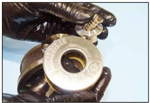
55. Remove the screw and the spring.
