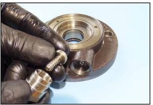
64. Assemble the oil retention valve with housing.
