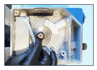
22. Place the cover plate and screw the cover of the suction felt.
